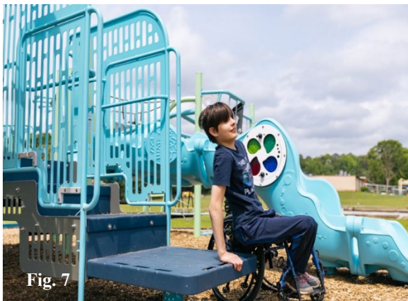
Fig. 7 - Example of child using transfer platform to transition from mobile device to platform.
