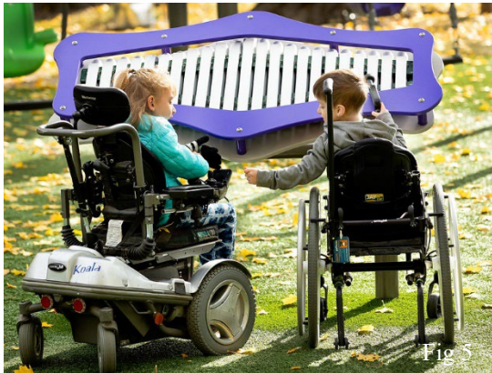
Fig. 5- Example of clear floor space in front of ground level component.
